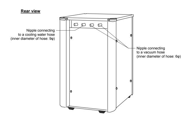
This equipment is used to collect the solvent in the rotary evaporator.
