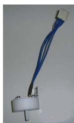
VR type pressure sensor for organic solvent
