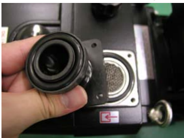
Photo-4: Set O-ring in its groove
