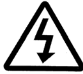
Danger!: High voltage
