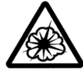
Danger!: Hazard of explosion
