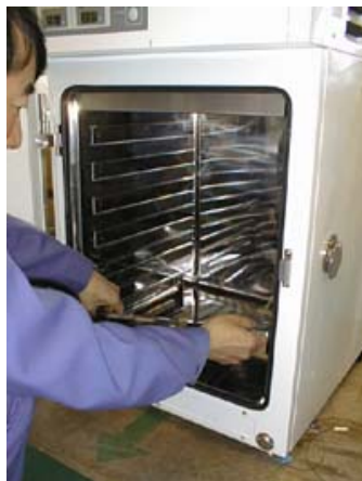
Photo 9: Insert the humidifier bat.
