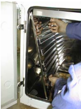
Photo 7: Press both left and right shelf poles into the wall of the bath.
