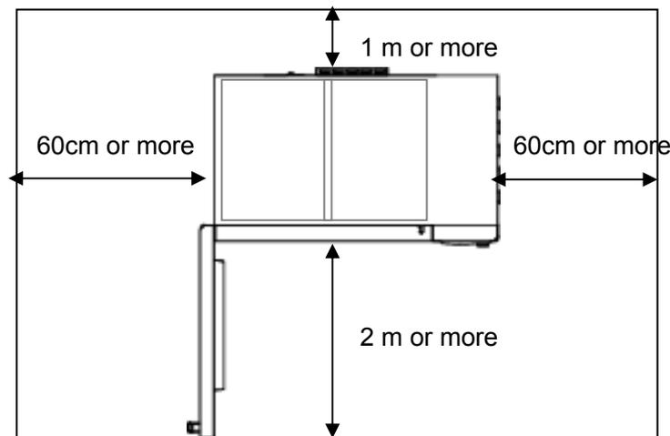
Make at least 2m of space on the ceiling (There shall be no lighting apparatus or other devices on the ceiling).
