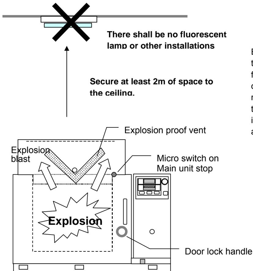
Explosion blast will blow up toward the ceiling. If there are fluorescent lamps on the ceiling, secondary disaster may result. Install the unit at a place that seems to be free of installations that might present a risk.
