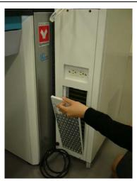
Simply pull the filter holding plate toward you which is held with magnets.
