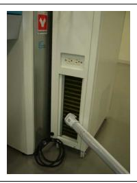
Remove dusts in the condenser fins with an electric cleaner.
