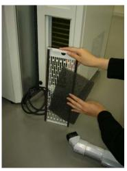
Filter is held with the filter fixing plate. Remove the filter and wash or remove dust with an electric cleaner with the filter attached.
