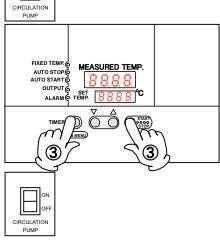
③To release lock, press the Sub menu key for four seconds.
