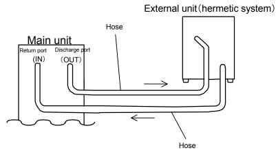
\*Attach a hose band and tighten it at the connecting point between the unit and the hose
