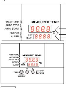
Turning the ELB on will display the starting screen for four seconds. Then the screen switches to the initial setting screen and each indicator shows the present in-bath temperature and the set temperature.
