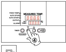
④ Select "off" with the ▼▲ keys and then press the Start/Stop key to release.
