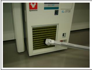
Remove dusts in the condenser fins with an electric cleaner.
