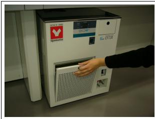
Simply pull the filter holding plate toward you which is held with magnets.
