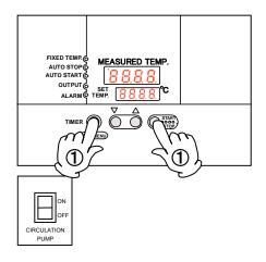
①Press the Sub menu key for four seconds. Then press the Sub menu key to select the characters  $\operatorname{Accm} \overline{\operatorname{\mathit{Hccn}}}$  that mean the accumulated time and press the Start/Stop key.
