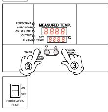
③To release power failure compensation, press the Submenu key for four seconds.
