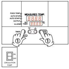
This function can be used when a power failure occurs to allow resuming operation at a state immediately before that power failure.
