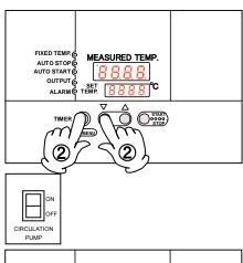
②The indication "off" comes on in the set temp screen. Turn this indication to "on" with the ▼▲ key to set the power failure compensation operation.
