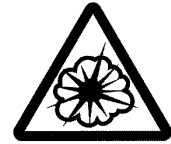
Danger!: Hazard of explosion
