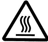
Danger!: High temperature
