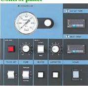
■ Inlet temperature, outlet temperature are displayed digitally. Condition setting dials and stage level control switch are located on the front panel for easy use.
